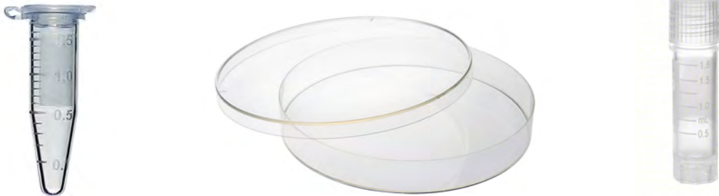
Fig 6: 1.5mL microfuge tube (left), 10mm Petri dish (middle), and 2mL cryovial (right).
